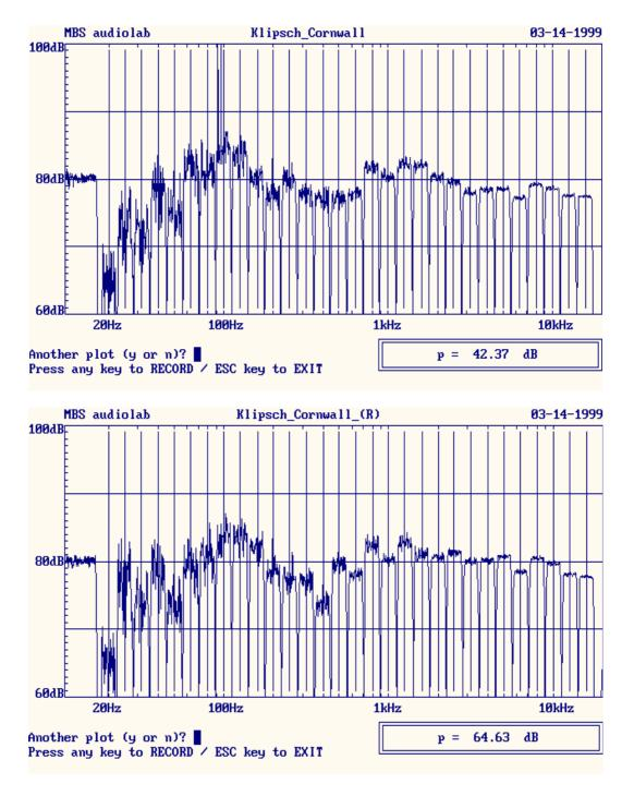
Frequency response is smooth from 25 Hz up to 20 kHz. A "deep" at 350 Hz is due to floor reflection (microphone was 1 m from front panel, and the acoustics in my quite reverberant room is not an easy problem) and a narrow resonance at 100 Hz is due to door (!) resonance.
