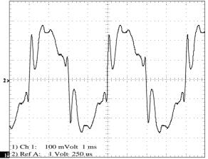
First picture shows 1002.27 Hz square wave signal as recorded on CTC CBS CD-1 test record (Track 16). Please note that even the shape which serves us as our input signal is not of ideal square wave at all.
