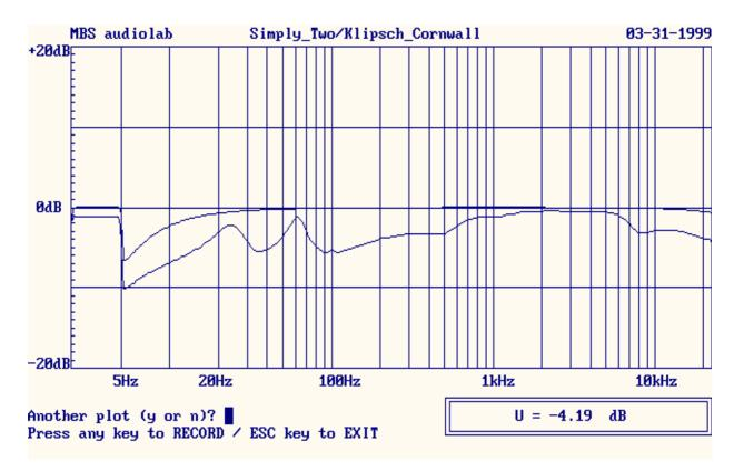
Similar plot was then obtained with Unison Simply Two pentode tube amplifier, set for lower "Feedback 2".
