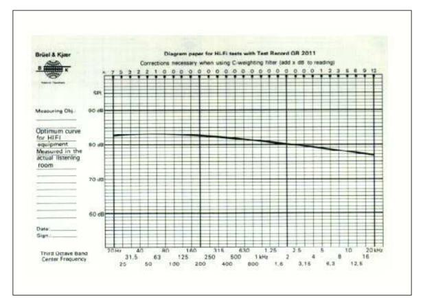
Simple explanation of this curve is that the best listening results can be expected when living room when actual frequency response of the particular loudspeaker corresponds to described curve. This curve could therefore be used as an "optimum", "calibration", "standard", "reference" or "flat" in any listening room loudspeaker evaluation.
