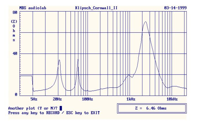
The lowest value is 5 Ohms at 20 and 100 Hz and the highest value is 75 Ohms. Nominal impedance corresponds to average "8 Ohms" value. But, according to tolerances given by well known German Hi-Fi standard DIN 45500 it might also be defined as "6 Ohms" as well.
