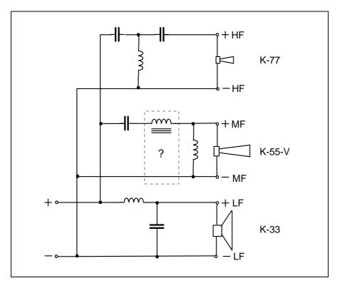
Klipsch Cornwall II crossover network (B600/6000Hz) schematic
