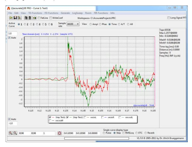
Several iterations with macro4 and testconvolution are required but still the result is not satisfying. In most cases only smaller values and thus less phase correction will help. The behaviour is not predictable, it is changing from room to room and from speaker to speaker.
