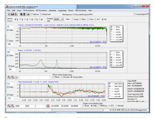
The example shows a single peak for left and right channel, left side with a higher frequency. The step response confirms these peaks.
